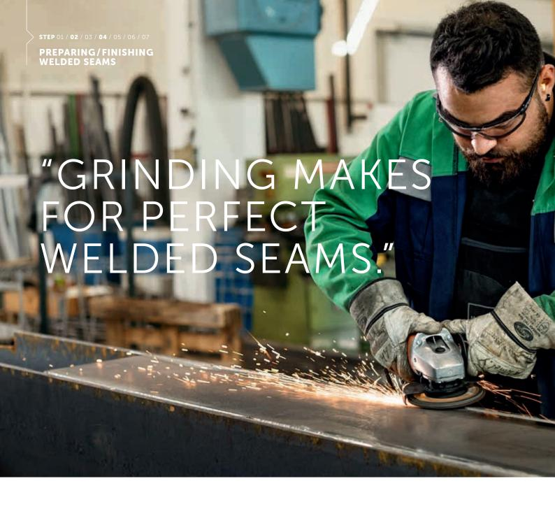
After chamfering with their bevelling machines, the professionals at Metallbau Perger prefer to move to angle grinders to grind down any remaining impurities, such as scale on the material surface. Grinding the surface can minimise welding errors, such as inclusions or incomplete fusion and therefore improves the quality of the welded seams.
