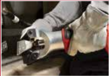
Auto distance control continuously measures distance & pressure
