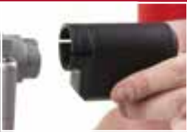
Retention nose pieces hold rivets in any orientation
