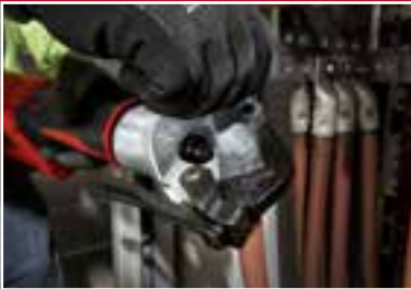
180° rotating head and easy access latch
