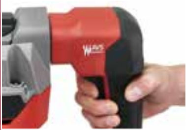
Large AVS back and side handle minimises vibration exposure
